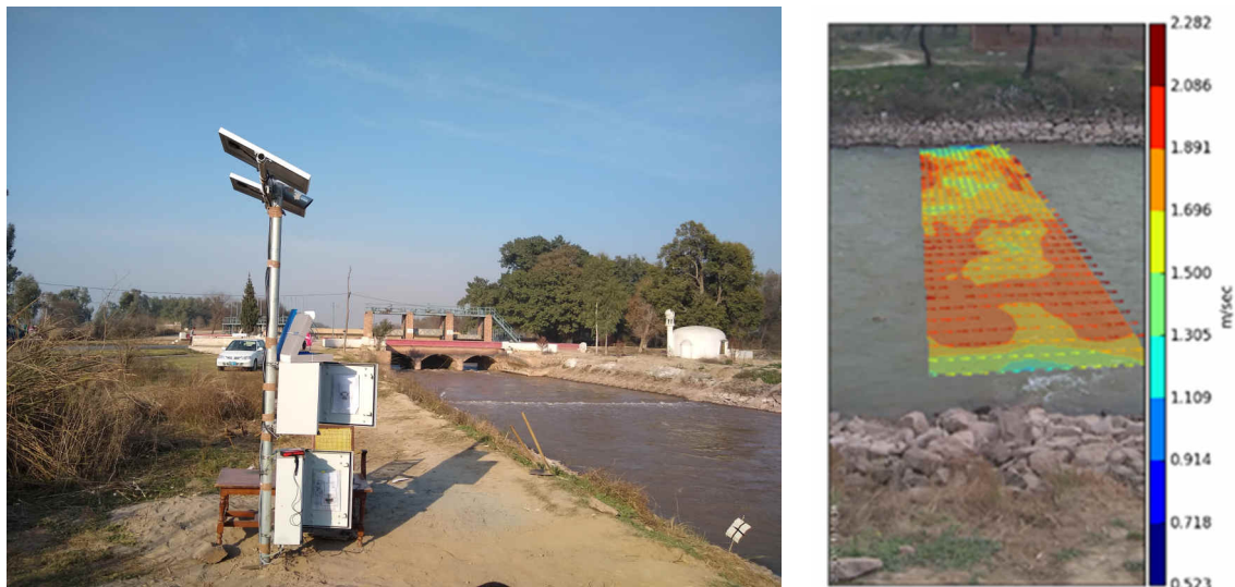
Figure 6.14: Optical discharge measurement station at Buralla branch (left) and measured Surface velocity distribution (right) © SEBA
