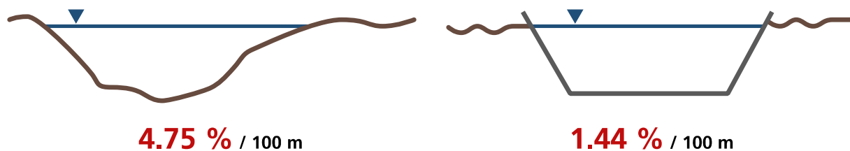
Figure 8.5: Visualization of mean losses in percent of initial discharge per 100 m from unlined (left) and lined channels (right).
