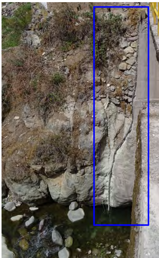
» Figure 2.5: Stream gauging station at Santa Rosa de Quilquichaca (3000 m asl): View on the installation at the right river-bank from the bridge above (the river flows to the left); the rectangle highlights the installation tube, which has a length of about 10 m (left). Cross-section and part of the river bed under the bridge, looking upstream (right). Pictures: S. Schroers.
