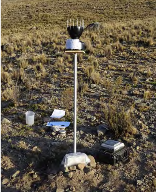
» Figure 2.4: Assessing soil hydraulic conductivity in the Lurín catchment using a hood infiltrrometer (left). Rain gauge RSN05 in San Damián district at 4455 m asl (right). Pictures: J. Bondy.
