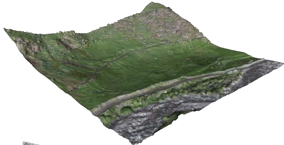
» Figure 2.7: Digital elevation model (DEM) of an area at the Lurín catchment (see Riese et al., 2020b) generated from an UAV, which is equipped with an RGB camera.
