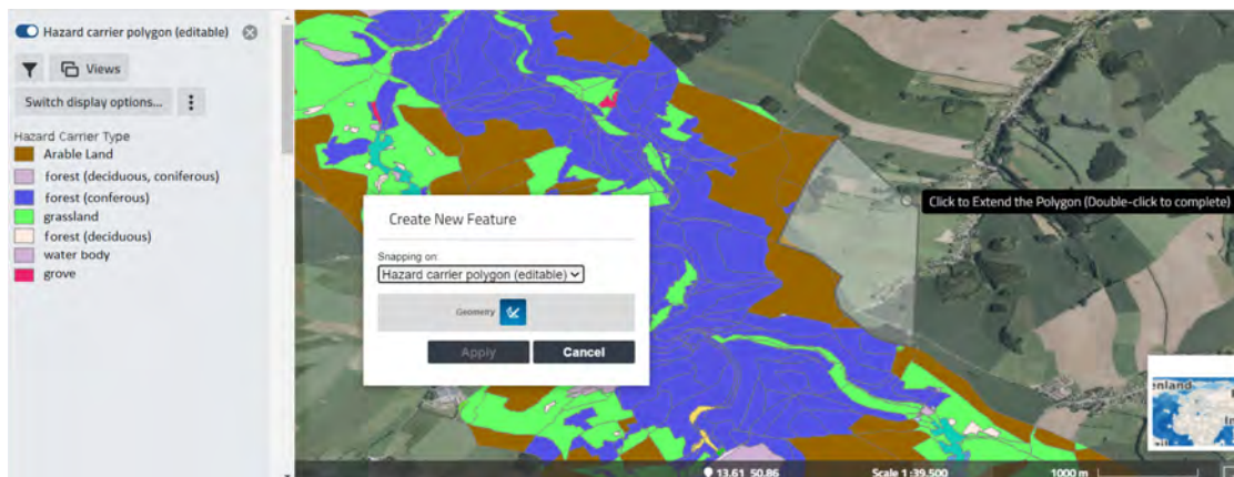
» Figure 2.15: Recording of hazard carriers in the map (test area Klingenberg, Germany).
