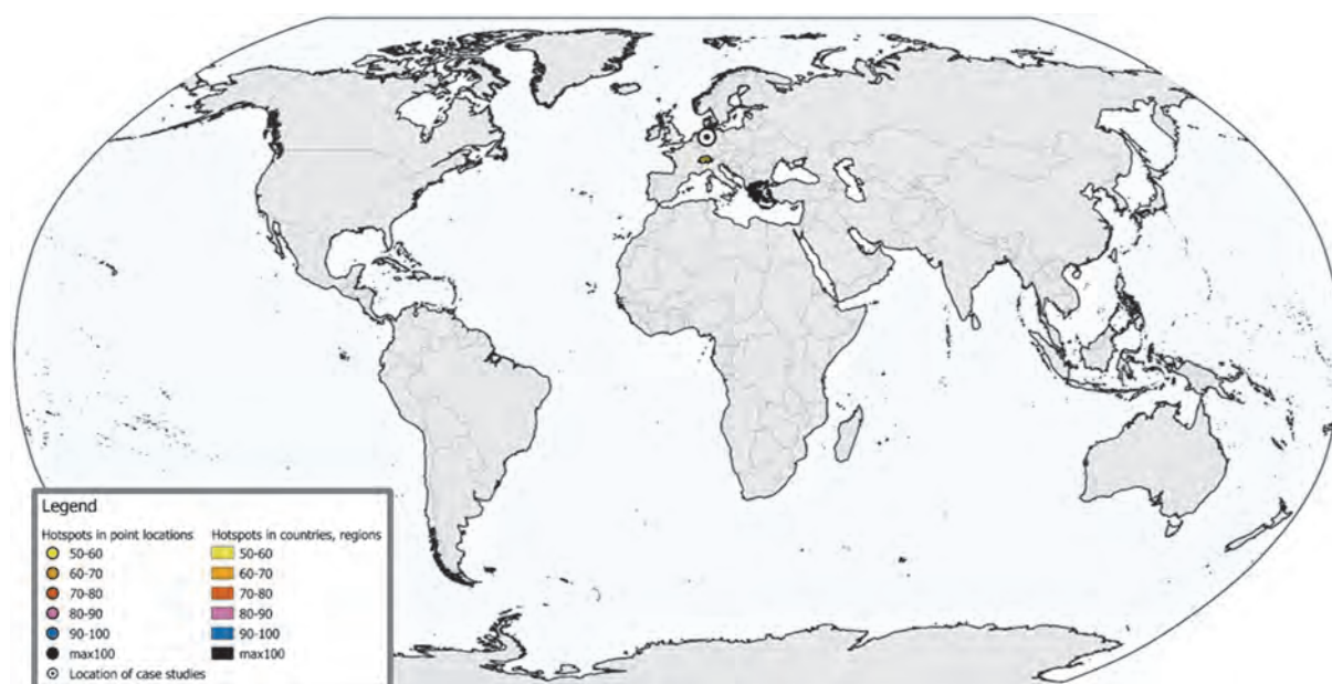
Figure 3-2: Hotspot analysis of the indicators WSF quan and WSF qual for case study 1 – the coal-fired power plant Heyden. For each indicator, single process results have been normalised using the median of all case studies. Results have been summarised per location per case study. Values greater than 100 have been set to a maximum value of 100. Any location with a value greater than 50, which equals a medium stress level on the scale from 0 to 100, is considered a hotspot. Global and rest-of-World (RoW) processes are excluded from the analysis. Their share in the total indicator results can be up to 65%. Processes that contribute less than 1% to an indicator result, respectively, are also excluded from the analysis.
