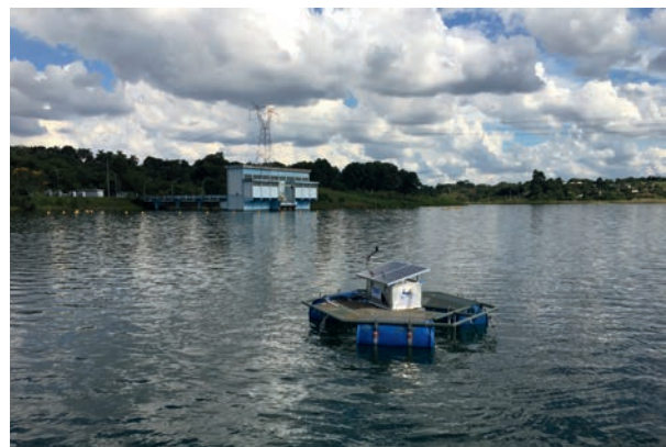
Measurement platform equipped with water quality sensors (foreground) and water extraction at the Passaúna reservoir (background)
