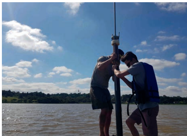
Two doctoral students from the Karlsruhe Institute of Technology (KIT) extract a drill core for sediment analysis
