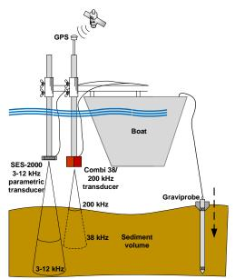
Fig. 1 Setup of the acoustic measurement system and application of the GraviProbe
