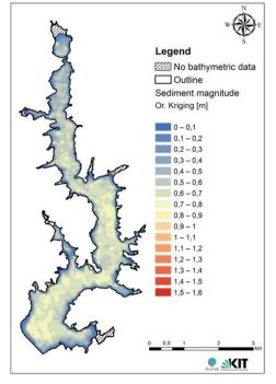
Fig. 3. Spatial distribution of sediment thickness in the reservoir from hydroacoustic measurements the sedimentation rate is larger than previously calculated from Sauniti et al. 2004 (up to 3 cm/year)
