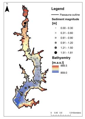
Fig. 2. Locations of GraviPrope measurements with sediment magnitude at the corresponding location, multibeam bathymetry in the background
