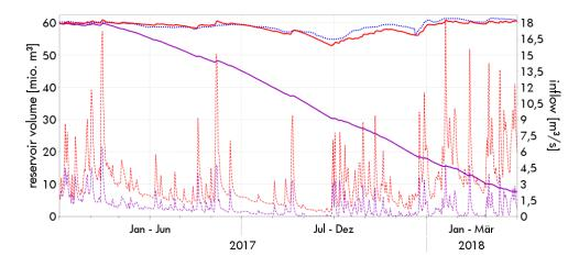
Figure 3: Comparison of two different simulations of the volume in Passaúna reservoir for the years The 2017/2018. versions differ only with respect to precipitation input (broken lines, right y-axis). In version 4, actual precipitation is reduced by 50%.
