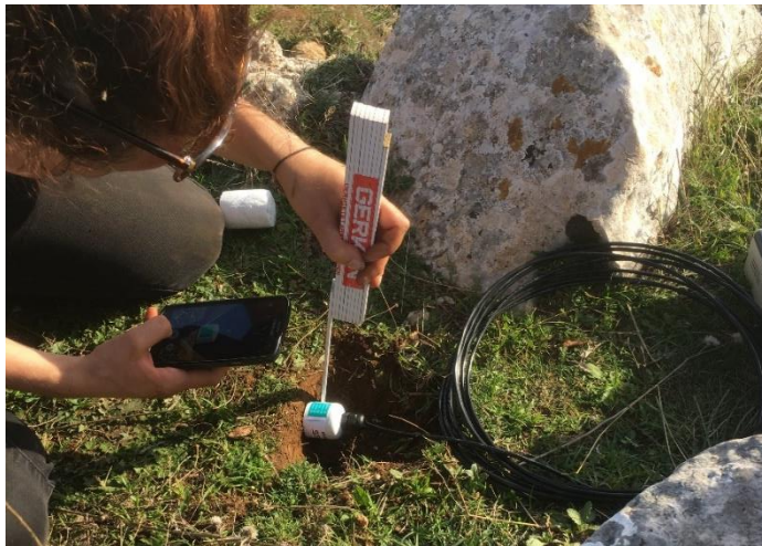
Soil moisture sensors (measuring depth: 10 cm)
